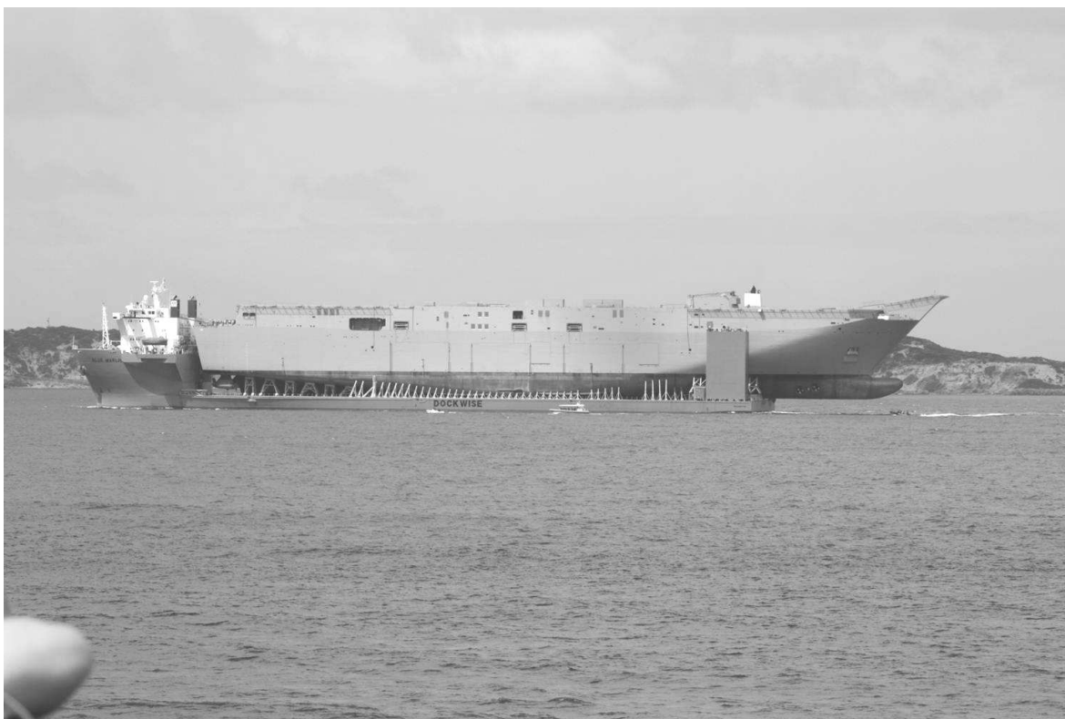
The hull of HMAS Canberra 3 was in Geelong Victoria in preparation for floating off of Blue Marlin on 22 October 2012.
