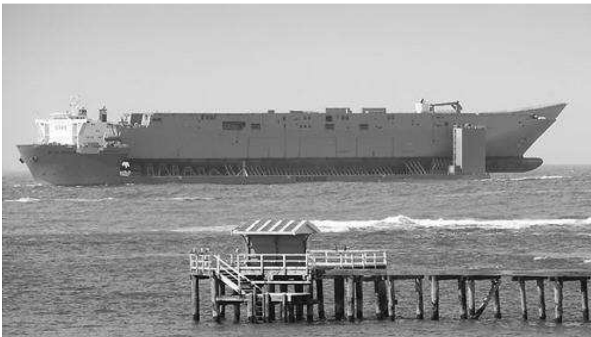
The MV Blue Marlin enters Port Phillip Bay on 17 October 2012 with the Hull of the future HMAS Canberra 3 onboard..
